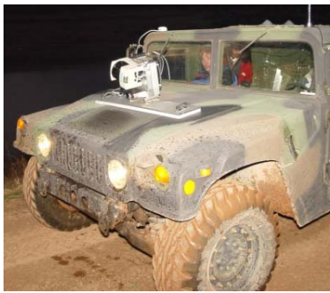
Fig. 3. A SIAB unit mounted on a HMMWV during the field tests described in Section V. A special mounting plate was designed to hold the unit on the hood of the vehicle and provide shock absorption.
