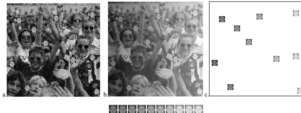
Figure 10: An original image was embedded with 10 occurrences of a pattern. a) Noise was added to the image at a level of 40 (see text). b. A gradient of illumination was added to the image. The 10 patterns as appearing in the image are shown below. c. All 10 patterns of varying illuminations were found. Five projections were required to find all 10 patterns.
