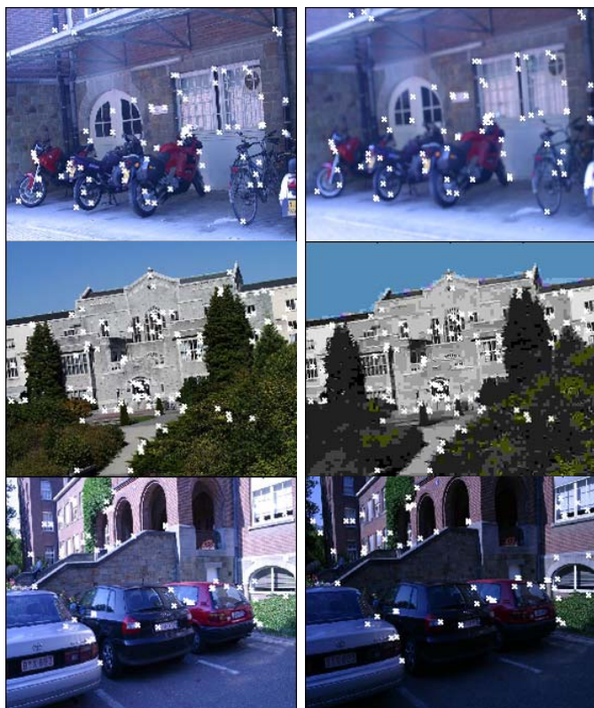
Fig. 7. Examples of photometric variations. Top row shows the matching results of image blur. There are 79 inliers. The second row shows the matching results of jpeg compression. There are 102 inliers. The third row shows the matching results of intensity changes. There are 68 inliers. All are correct.
