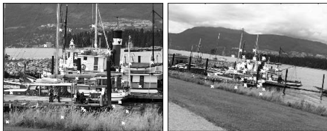
Fig. 5. Example of scale and rotation changes. The two images are frames of "boat" from Oxford Univ. There are considerable rotation and scale changes between them. There are 47 matches. All are correct.
